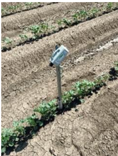
Canopy Temperature Sensor similar to this have been installed at 'Cleveland'
