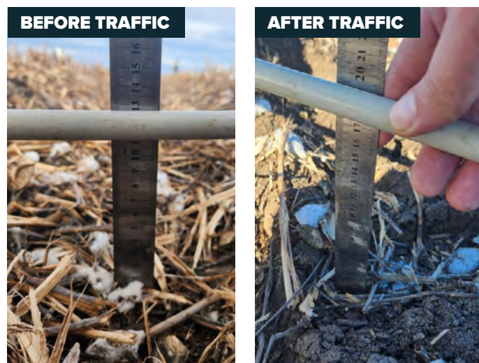
Picture 1. shows the change in wheel rut depth after cotton picker traffic on a wet soil at Narrabri.
