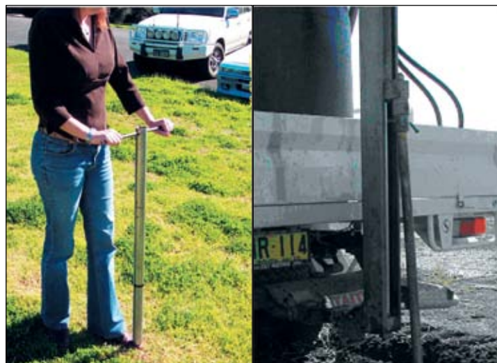
Hand cores are suitable for up to sampling up to 30 cm deep while vehicle mounted coring tubes are used when greater sample numbers and sampling depth is required.
