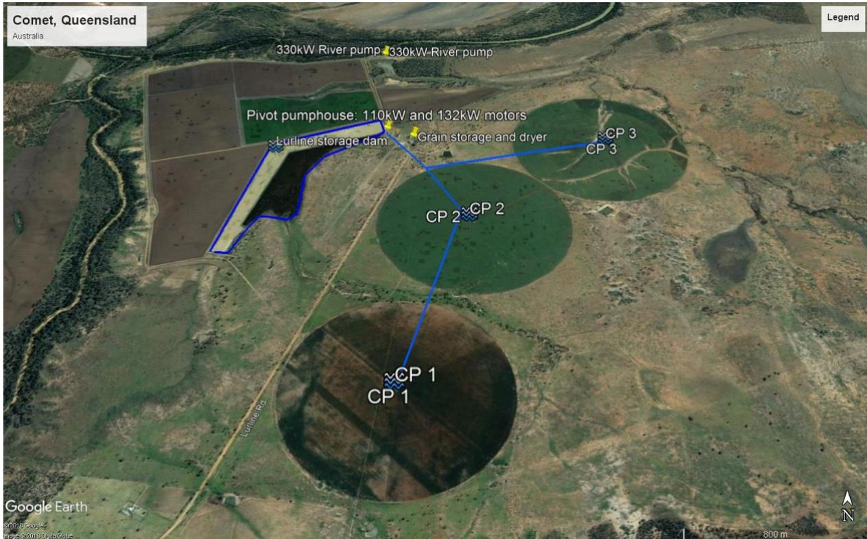
FIGURE 3: CASE STUDY FARM MAP SHOWING THE IRRIGATION LAYOUT AND GRID-CONNECTED LOADS (YELLOW PLACEMARKS). MAP IMAGE COURTESY GOOGLE EARTH.
