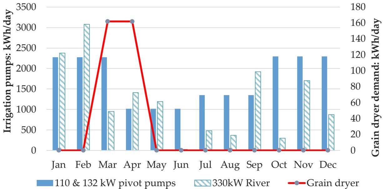
**FIGURE 5: MONTHLY AVERAGE ENERGY DEMAND FOR EACH SITE: RIVER PUMP (SITE A), PIVOT PUMP HOUSE (SITE B), AND GRAIN DRYER (SITE C).**
