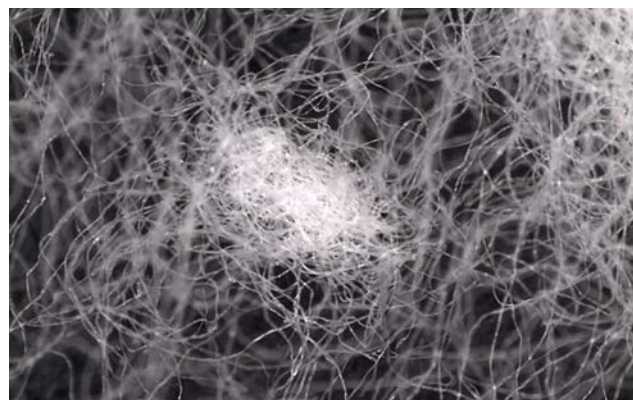
FIGURE 7 Image of a fibrous nep
