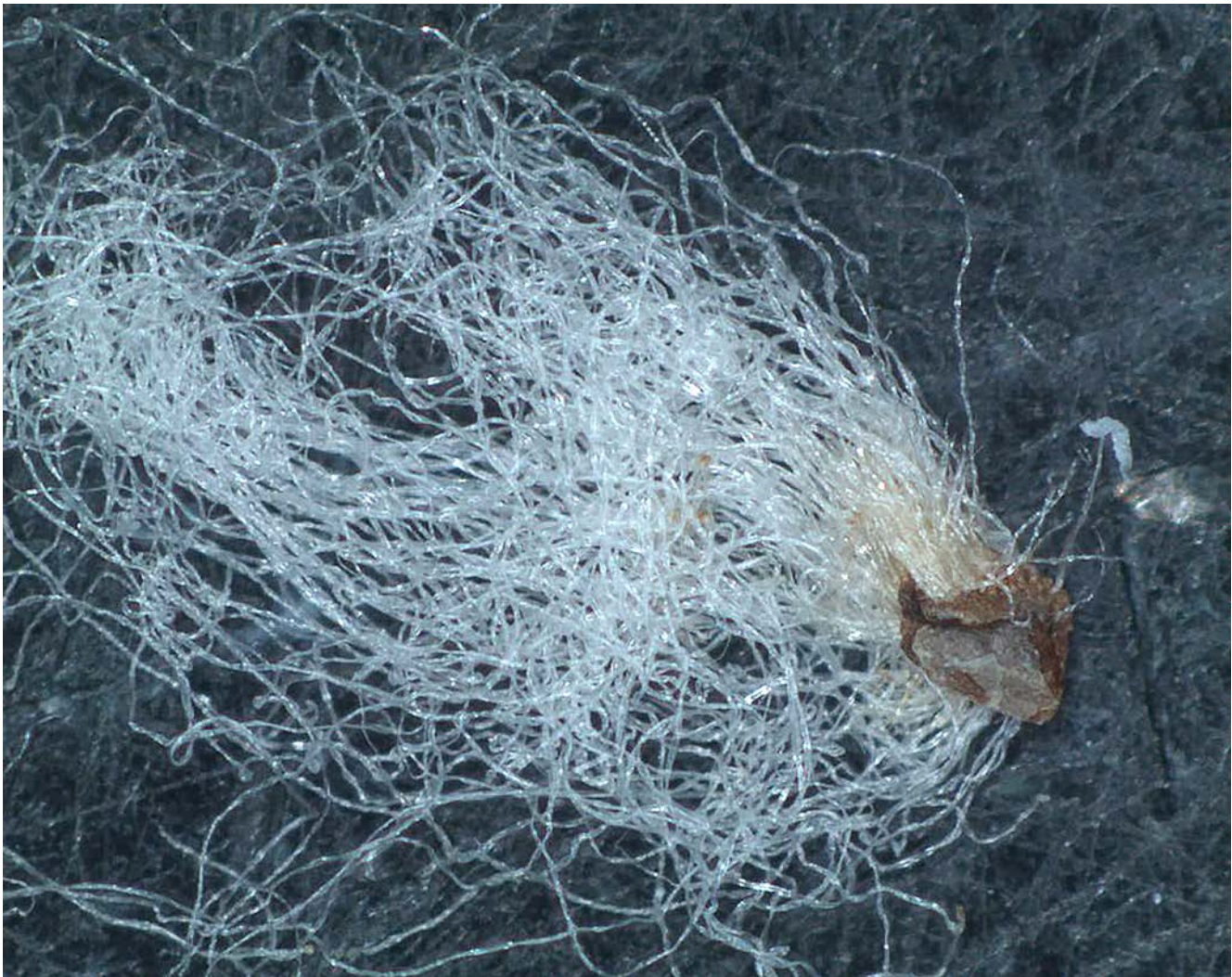
FIGURE 8 Image of a seed-coat fragment nep
