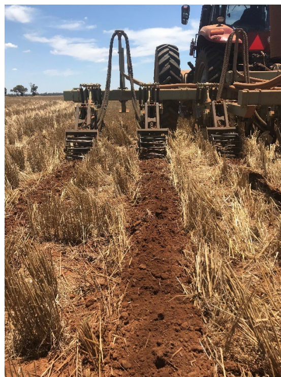
Fig 3 – strip tiller preparing the bed for planting into wheat stubble crop.
