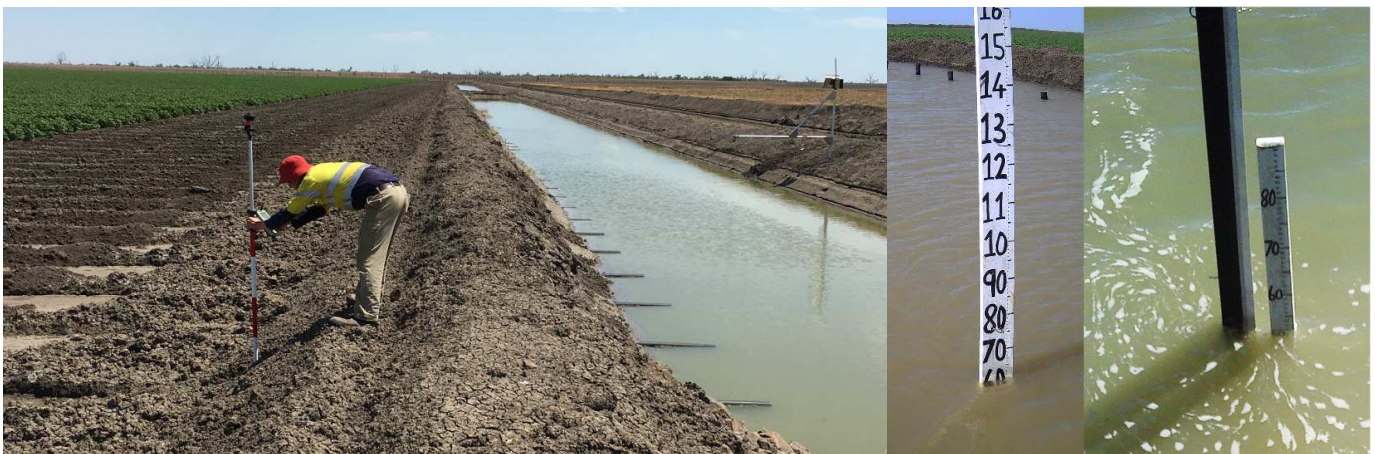
Figure 2 : (a) measuring pipe outlet levels (b) sample images from smartphone cameras
