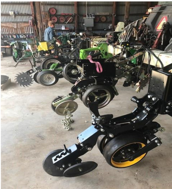
Planter Bar under construction.
