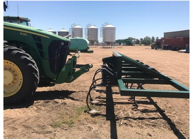
Front mounted chisel plough At “Waverley”
