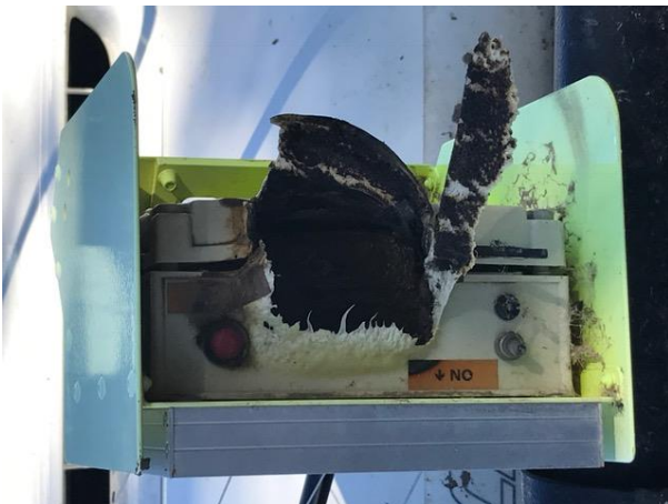
The weather station at "Miralwyn" had a slight battery malfunction.
