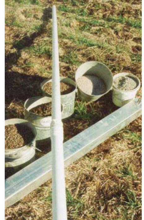
Figure 3 – Materials to install a shallow monitoring piezometer
