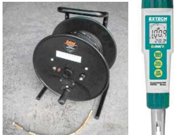
Figure 4 – Example of water level dipper and pocket sized salinity EC meter.
